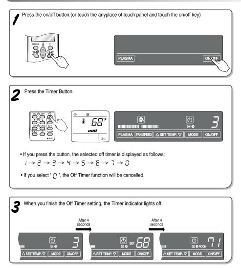
During off-timer operation if you press the Timer Button, the rest time will be displayed.
